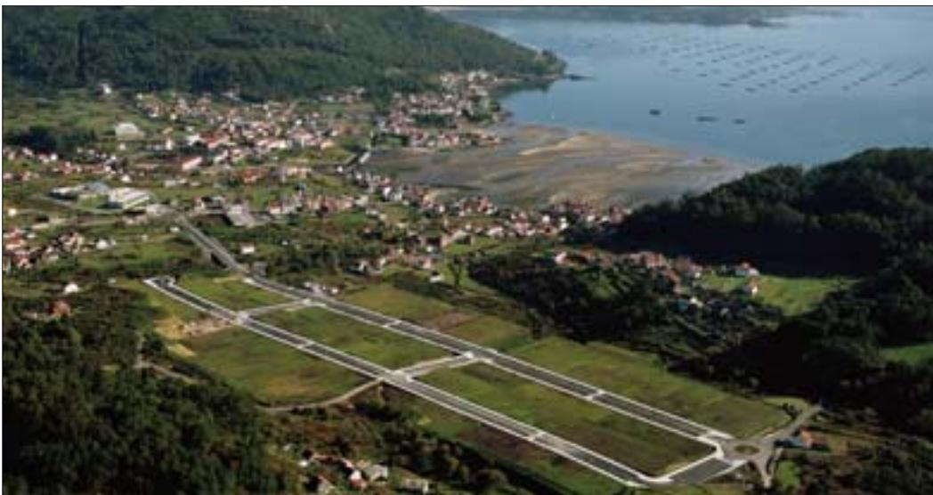
Two longitudinal and two transversal roads, with a 23 meter-section were built, plus two 3.5 meter-wide lanes, parking facilities and two 3 meter-wide sidewalks. A traffic circle, 800 meters-long and 11 meters wide, from the AC-400 road provides access to the business park.
